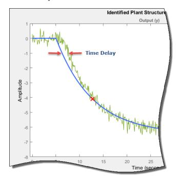
To add a transport delay to the estimated plant model, in the **Plant Structure** section, check **Delay**. A vertical line appears on the plot, indicating the current value of the delay. Drag the line left or right to change the delay, and make further adjustments to the system response by dragging the red x.
