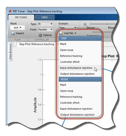
For example, to observe the closed-loop step response to disturbance at the plant input, in the **Step** section of the **Add Plot** menu, select **Input disturbance** rejection. The disturbance rejection response appears in a new figure.
