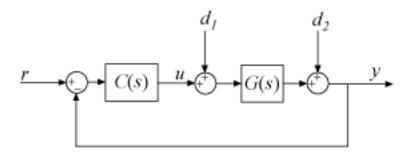
For 2-DOF PID controller types such as PI2, PIDF2, and I-PD, the software computes responses based upon the following architecture:
