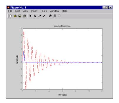
**Comparison of Open- and Closed-Loop Impulse Response**
