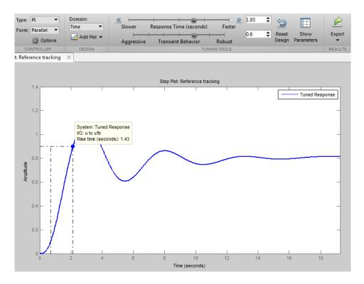
Moving the **Response time** slider far enough to meet the rise time requirement of less than 1.5 s results in more oscillation. Additionally, the parameters display shows that the new response has an unacceptably long settling time.
