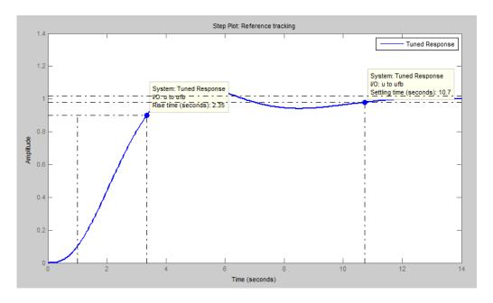
The initial PI controller design provides a rise time of 2.35 s and settling time of 10.7 s. Both results are slower than the design requirements.
