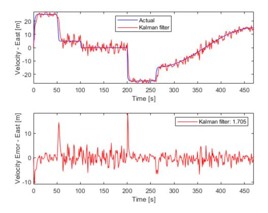
The legend on the error plot shows the east velocity estimation error  $||\dot{x}_e - \dot{\hat{x}}_e||_1$  normalized by the number of data points.
