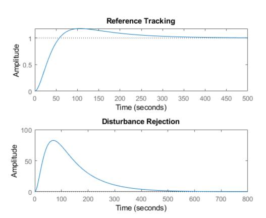
By default, for a given bandwidth, pidtune tunes the controller to achieve a balance between reference tracking and disturbance rejection. In this case, the controller yields some overshoot in the reference-tracking response. The controller also suppresses the input disturbance with a somewhat longer settling time than the reference tracking, after an initial peak.
