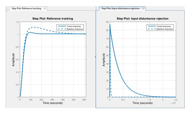
The PIDF controller tuned with reference-tracking focus is displayed as Tuned response (solid line). The plots show that the resulting controller tracks the reference input with considerably less overshoot and a faster settling time than the balanced controller design. However, the design yields much poorer disturbance rejection.
