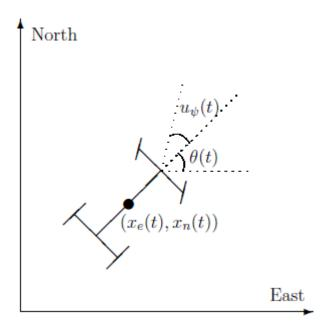
$x_e(t)$  and  $x_n(t)$  are the vehicle's east and north positions from the origin,  $\theta(t)$  is the vehicle orientation from east and  $u_{\psi}(t)$  is the steering angle of the vehicle. t is the continuous-time variable.
